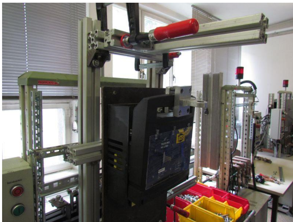
Photo 7: Test object TES-1/800 after the verification of the strength of actuator mechanism
