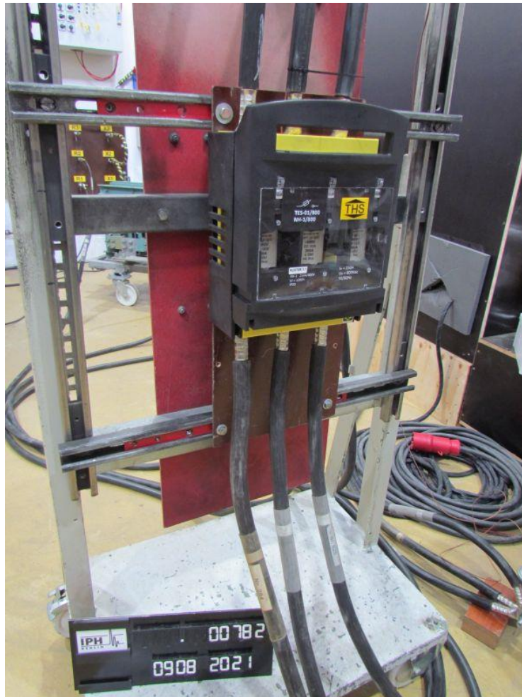
Photo 10: Test object TES-1/800 during temperature-rise verification
