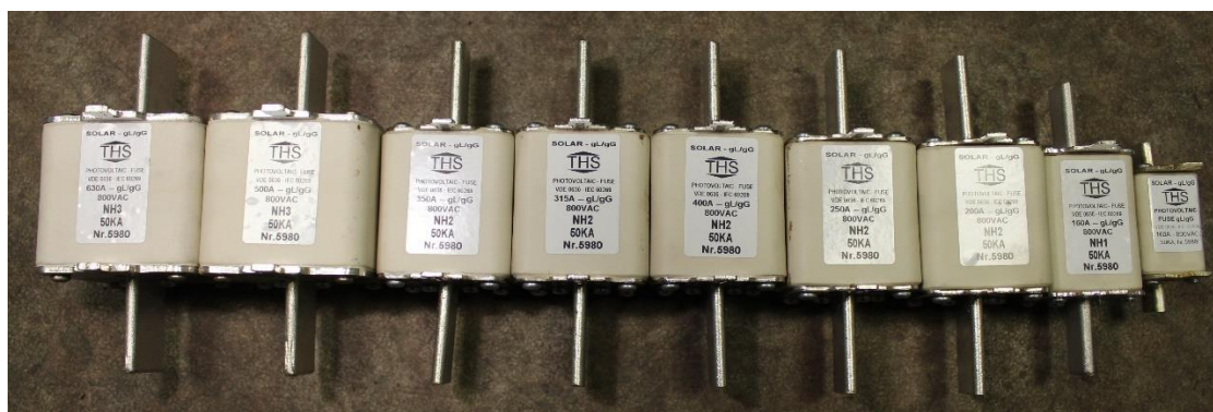
Photo 2: Fuses after all tests, rating plates
