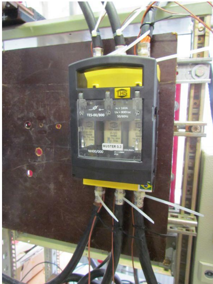
Photo 9: Test object TES-00/800 during temperature-rise verification
